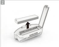
• Reinsert the high performance filter into the filter compartment. Close the compartment.
